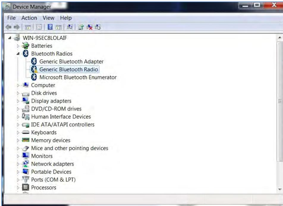
*Note: If you can't see any Bluetooth options in the list, make sure Bluetooth is switched on on your PC/laptop. If you can't see Generic Bluetooth Radio, your PC is not connected to the car kit control box.*
